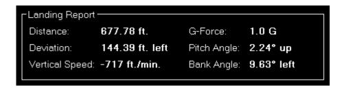
After the approach has been completed and the aircraft is landed, this landing report shows detailed
