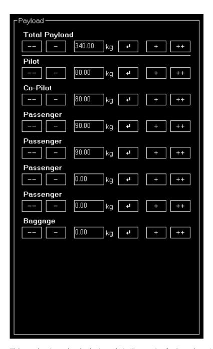
This payload section is designed similar to the fuel section: All payload stations are listed and the load of each payload station can be adjusted by clicking on the appropriate button or entering a specific value manually.
