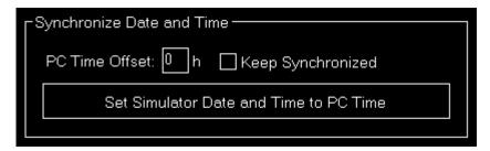
There is also the option to synchronize the simulator date and time with the one of the computer, optionally with a certain time offset.
