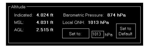
In the altitude section the current indicated altitude, the altitude above mean sea level (MSL) as well as the altitude above ground level (AGL) is displayed.
